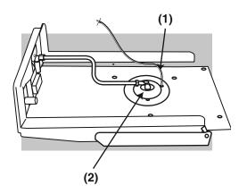
Make sure wire is connected between the igniter and electrode. Spark should be a white/blue color, not yellow.
